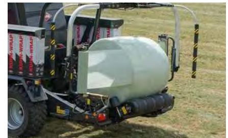
Switches to conventional wrapping for 100% film coverage.
