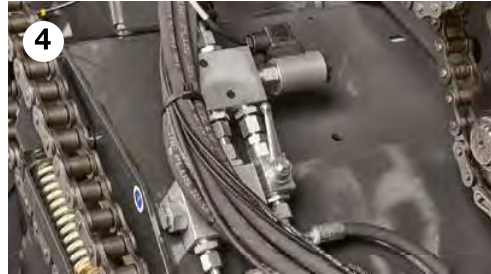
4 Separate knife / DROPFLOOR controlled from the tractor cab
