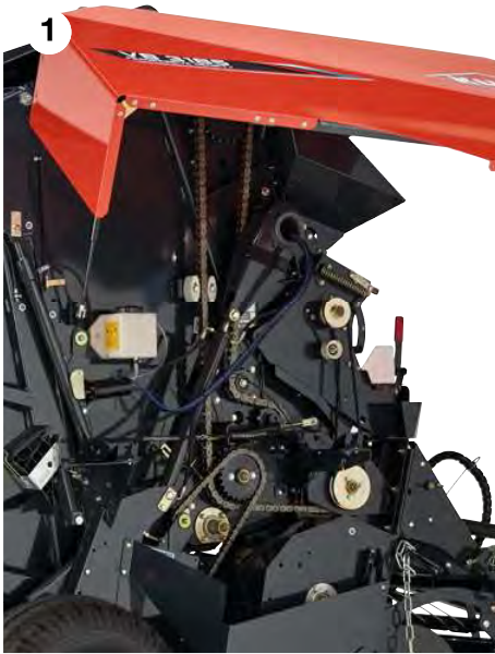
Robust driveline with high quality IWIS chains
