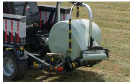
Further wrapping of the cylindrical surface of the bale until approximately 80% is covered.
