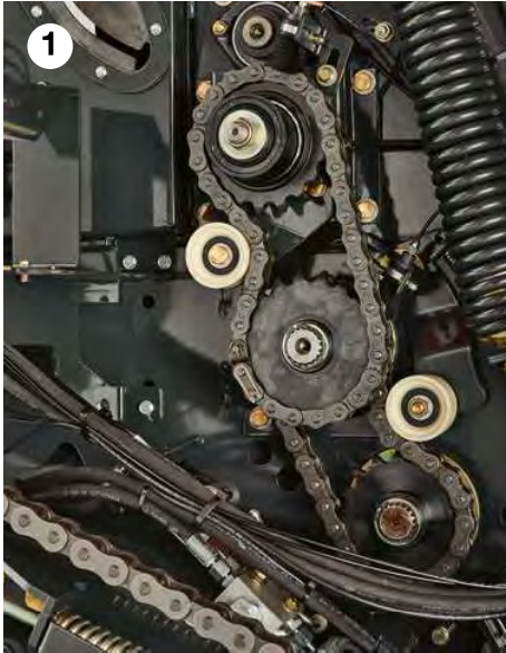
1 Second belt driven roller guarantees a secure belt drive in all crop conditions
