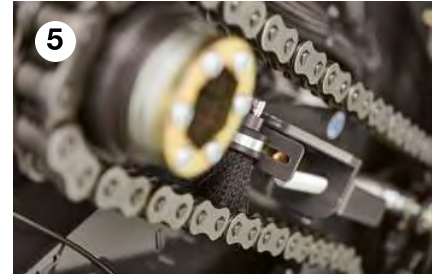
5 Sturdy and wide oil brushes on the chains ensure perfect lubrication
