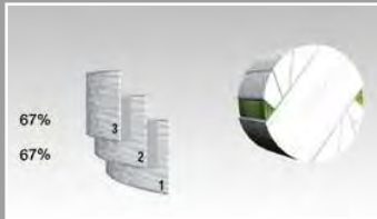
The bale is covered with 3 layers at 67% overlap.
