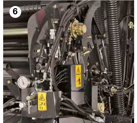
Proportional valve for in-cab density control
