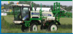
The AR2000 is a very nimble and compact machine, with a shorter chassis giving an extra-tight turning circle. Ideal for smaller or odd-shaped fields.
